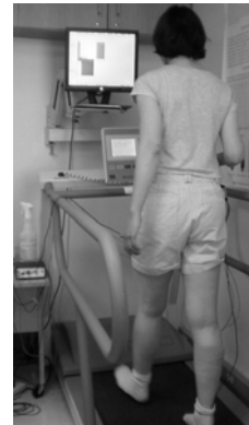
Figure 1. Experimental set-up with subject walking on treadmill watching screen for visual biofeedback.
