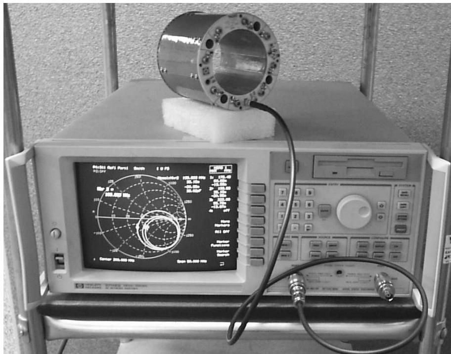
Figure 3-20 Network analyzer with the MRI RF coil attached.
