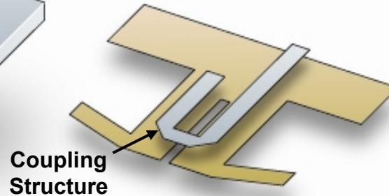
**Slot Cut in Waveguide**
