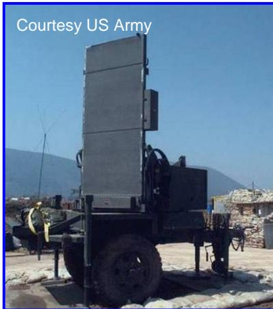
**Mechanical Scanning Antenna**
