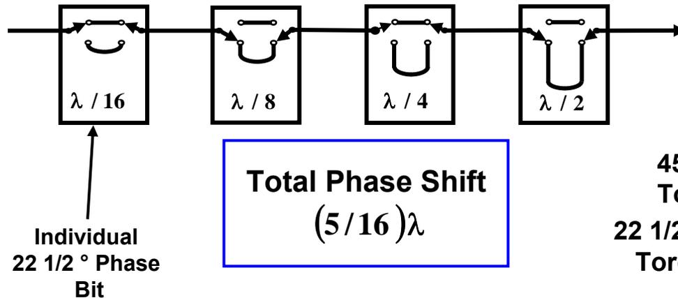
Four Bit Latching Ferrite Phase Shifter
