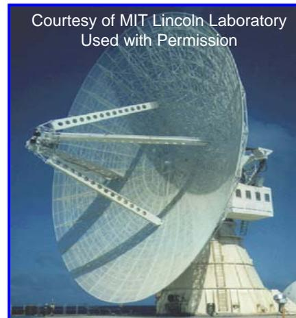
**Hybrid Mechanical and Frequency Scanning Antenna**
