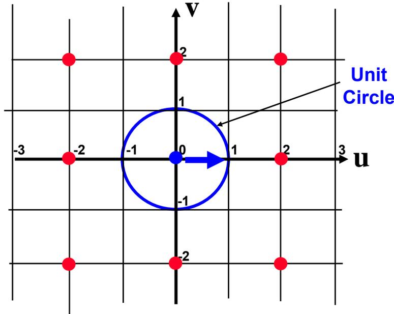
$$\text{Beam Scanned } \phi = 0^\circ, \theta = 90^\circ$$
