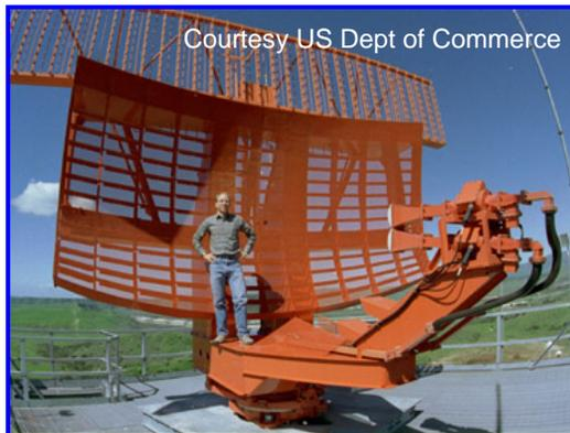
**Mechanical Scanning Antenna**
