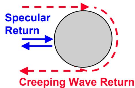
Radius of sphere is equal to the radar wavelength
