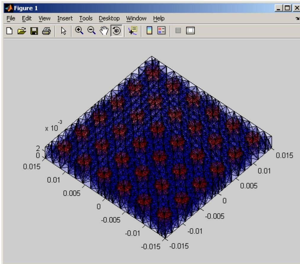
Fig. 1.15. The textured dielectric substrate.
