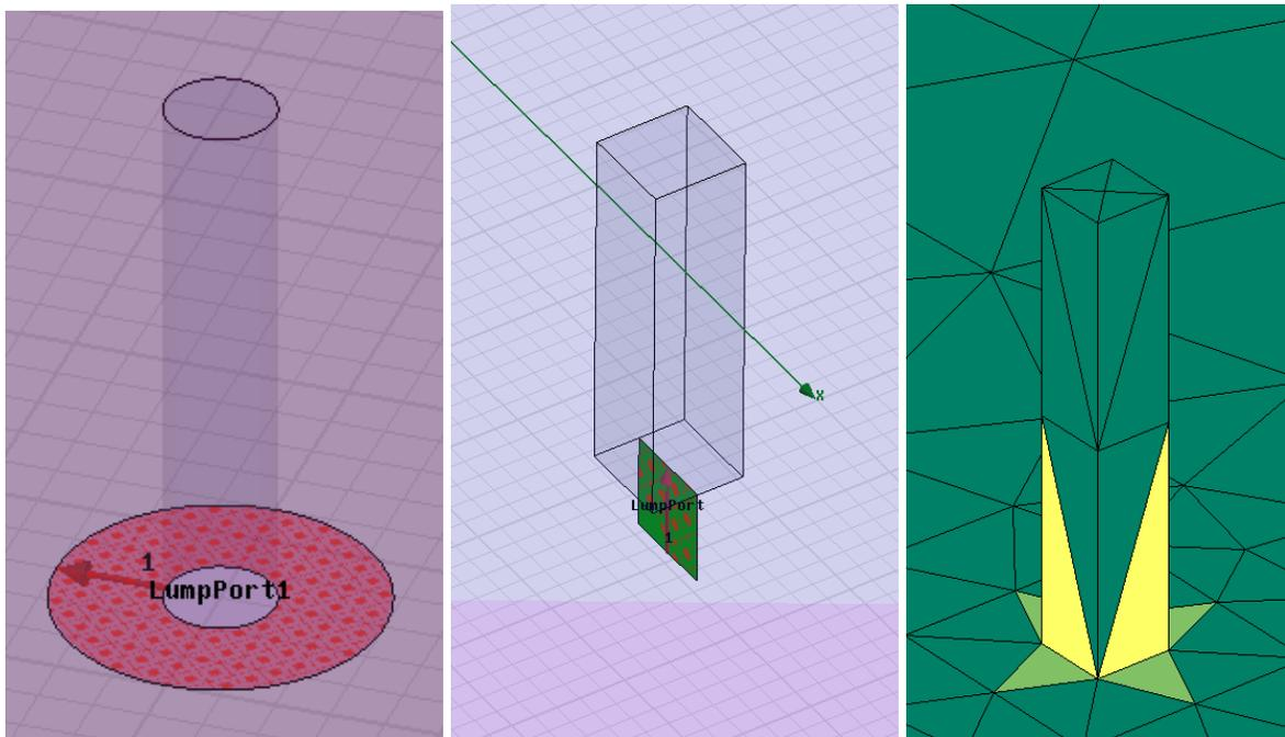
Fig. 1.13 Two feed models used in Ansoft HFSS solutions. Left – disk gap; center – voltage gap between the feed and the ground plane. The MoM voltage gap feed for the bottom edges of the metal column (two basis functions per edge) is shown on the right.
