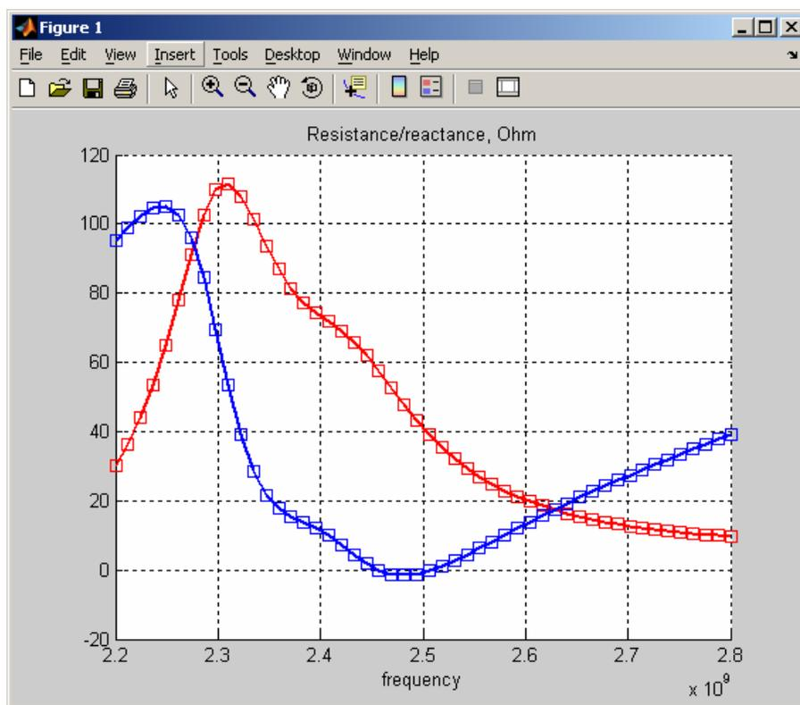
Fig. 1.7. Antenna input impedance. Reactance (blue) crosses zero at approximately 2.45 GHz.
