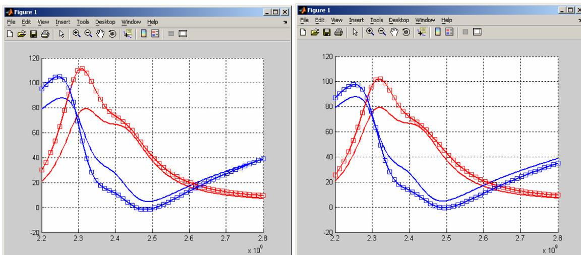
Fig. 1.12. Input impedance for the mesh with 1780 unknowns (left) and 4898 unknowns (right). The Ansoft HFSS solution is given by solid curves.
