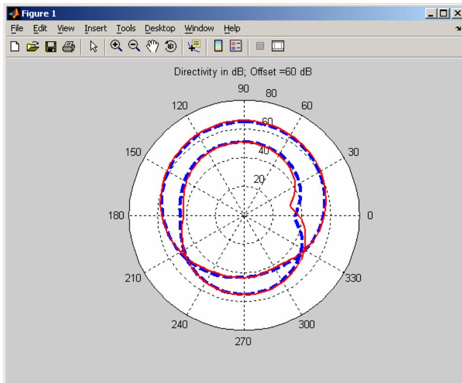
Fig. 1.9. Absolute directivity of RHCP (higher at zenith) and LHCP (higher in the back lobe) in the xz-plane of the patch antenna at 2.40 GHz. The corresponding Ansoft HFSS solution is shown by dashed curves. Note the offset marked in the figure title.
