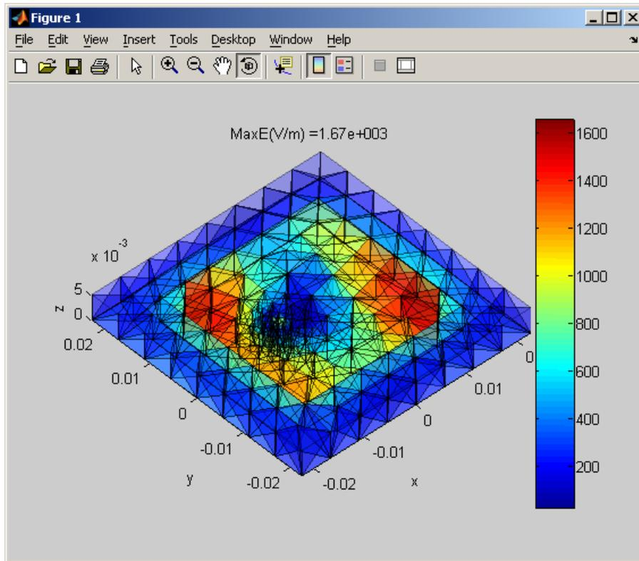
Fig. 1.10. The GUI output for the electric field in the dielectric (the magnitude of the dominant vertical component) within the patch antenna at 2.40 GHz.
