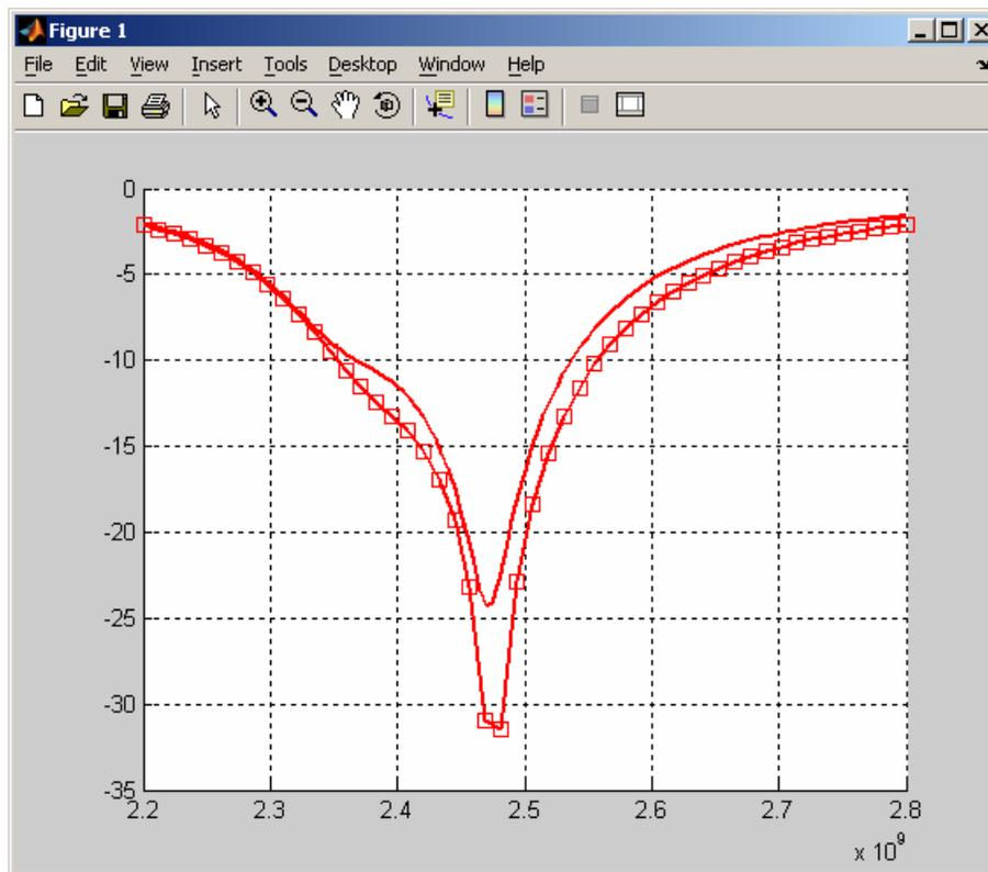
Fig. 1.8. Antenna return loss (squared curve) and the return loss predicted by the Ansoft HFSS solution with approximately 20,000 tetrahedra (solid curve). Note that MATLAB plots the negative value of the return loss.
