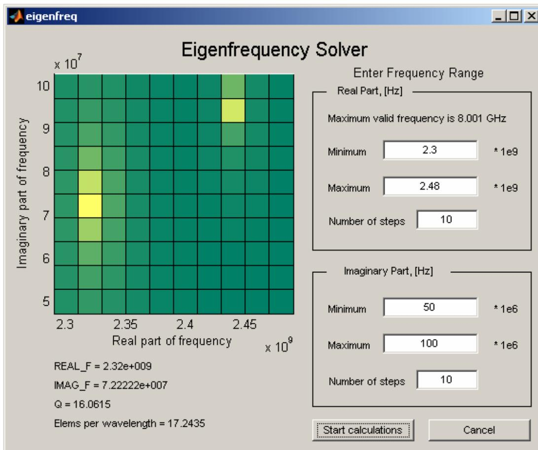
Fig. 1.11. The GUI output for the direct eigenmode solution for the patch antenna cavity (with the feed removed). The light dots in the plane of complex frequency indicate two close resonances.
