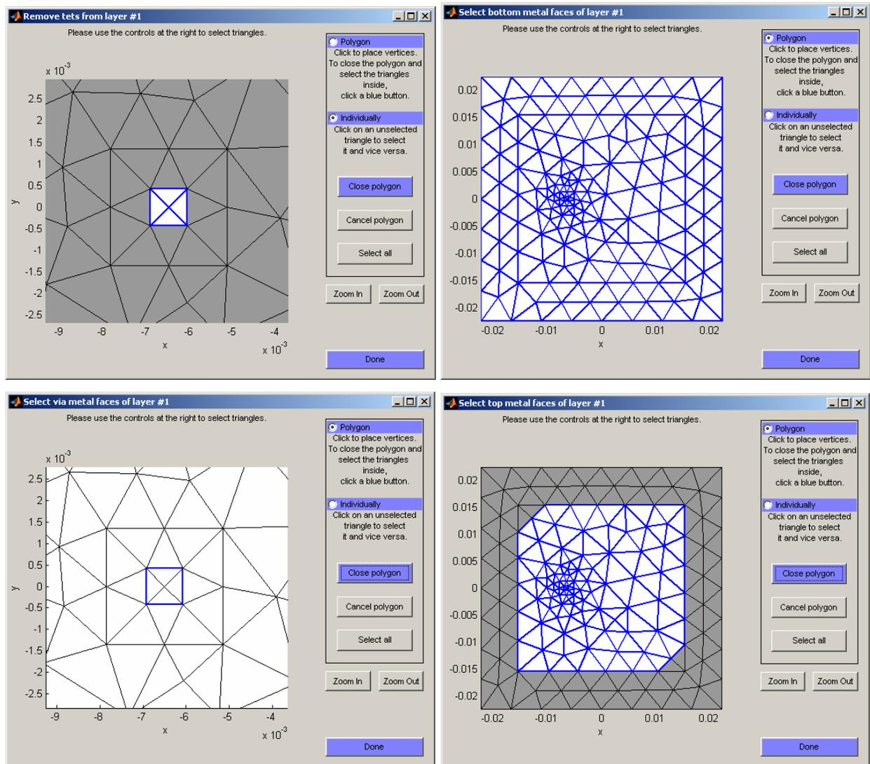
Fig. 1.5. Selection operations used to create the patch antenna mesh. Top left: selection of tetrahedra to be removed from the mesh (feed column only). Top right: selection of the ground plane. Bottom left: selection of the via edges and the feeding edges. Bottom right: selection of the patch.
