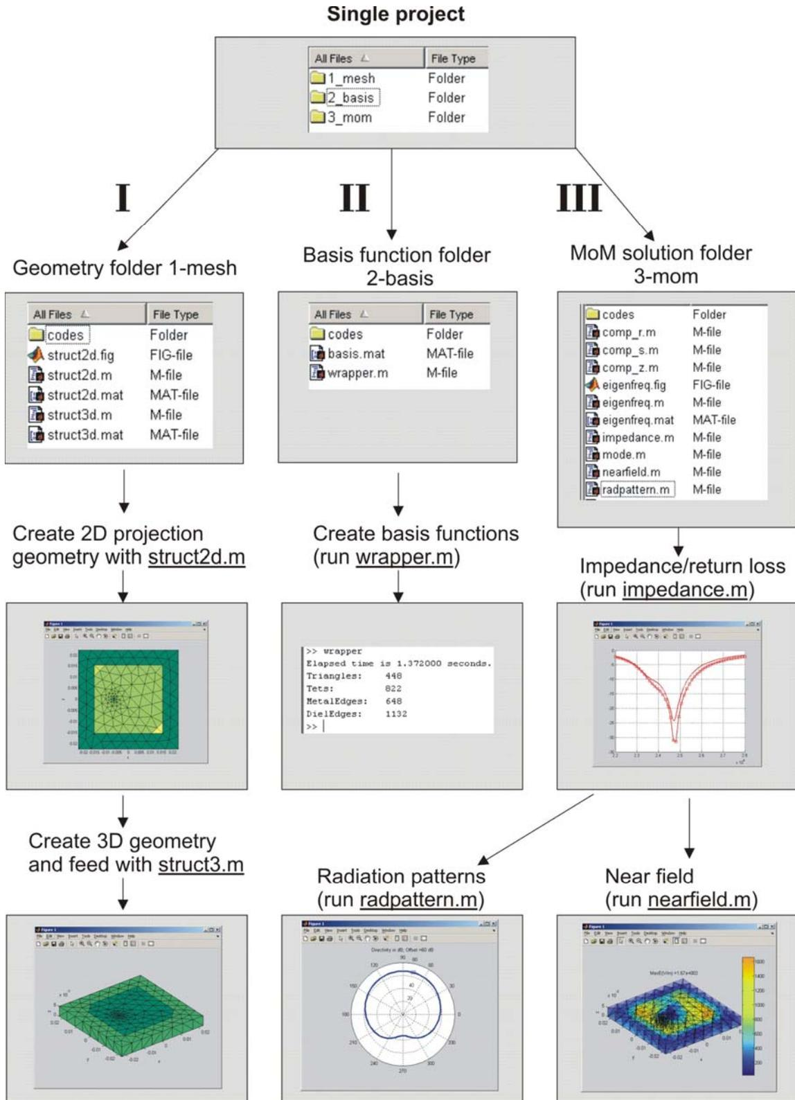
Fig. 1.1. Quick execution flowchart.
