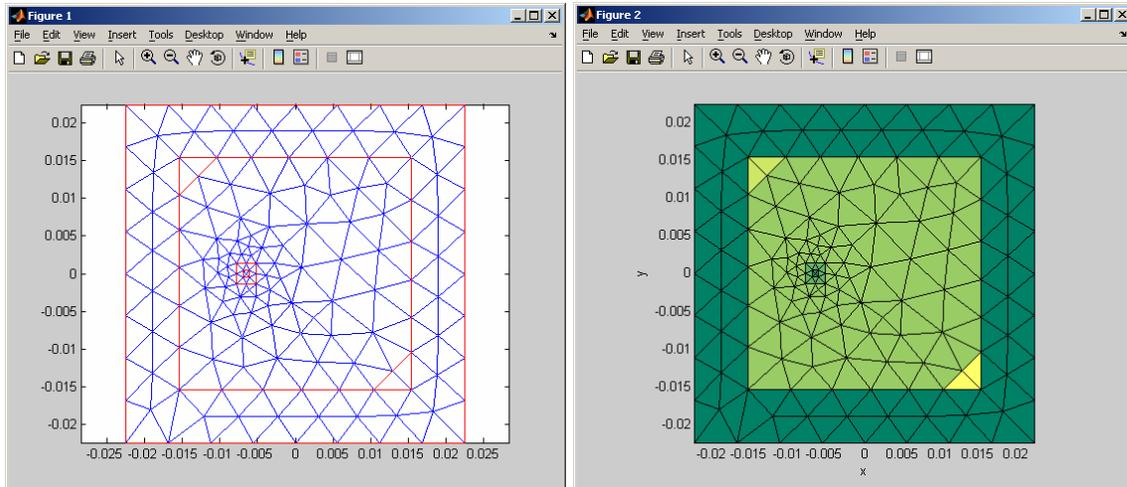
Fig. 1.3. View (left) and Accept (right) mesh screen. The surface mesh includes a ground plane shape and a polygonal patch antenna shape, with the feed position rectangle, which are both specified in the GUI in Fig. 1.2. Note that the `border` option in Fig. 1.2 is turned off. Different colors in Fig. 1.3 – right indicate different subdomain numbers used in the PDE toolbox.
