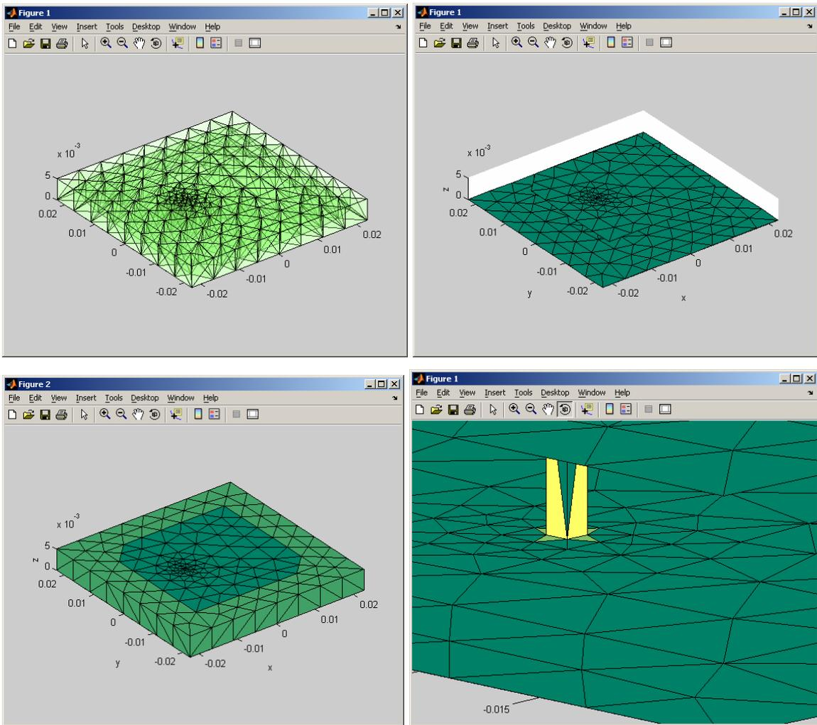
Fig. 1.6. Patch antenna mesh inspection using GUI `view3d.m`. From top left to bottom right: tetrahedral mesh, metal mesh, dielectric/metal mesh, feed column.
