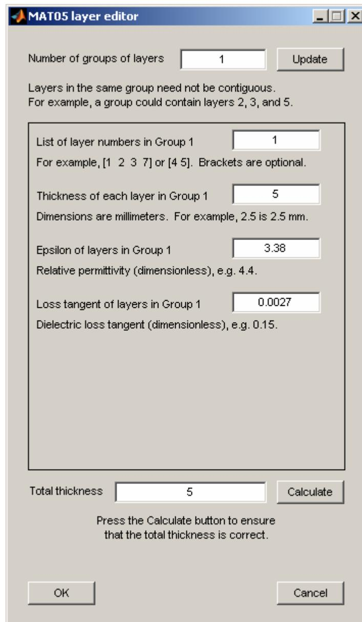
Fig. 1.4. Layer partitioner GUI `layers.m` – specifies parameters for separate layers of tetrahedra. The present GUI includes one layer and one group of layers.
