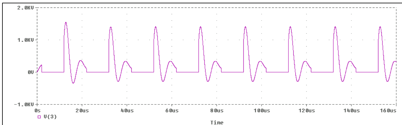
Figure 14: Voltage Across Switch (w/ snubber)
